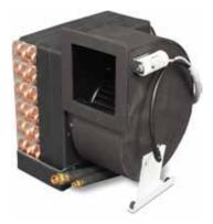
Compact EBE split evaporators for boats are draw-through, ductable cooling units with reversecycle heating. Featuring a rotatable, high-efficiency permanent split capacitor (PSC) blower in which the motor is concealed, EBE series evaporators are available in capacities from 6K to 36K BTU/hr. EBHE units have electric heat.
